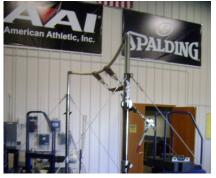
far, it's all good, but when that rail flexes, the distance from end to end must decrease because the bar does not have any end to end elasticity. Therefore, in order for the bard to flex, and the ends to come in, the uprights (vertical supports) must move in, forward, or back depending on which direction the bar is flexing. The uprights are anchored by steel cables which also do not stretch so they just transfer the force to the tie down that is connected into the floor anchor.
